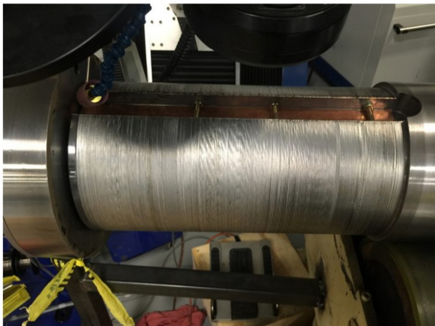
Shaft almost done welding. Note the small area on the left end of the diameter that has not been welded yet.
